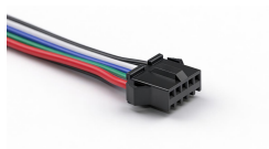
FC-5P-20 Female SM connector with 0.66ft (20cm) cable, 5pin, IP20, Dry, 22AWG
