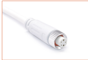
FCW-5P-67 Female connector, 0.98ft (30cm) white cable, 5 pin, IP67, Wet, 22 AWG
