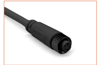
FCB-5P-67 Female connector, 0.98ft (30cm) black cable, 5 pin, IP67, Wet, 22 AWG
