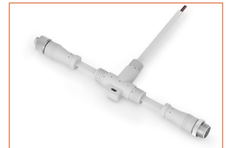
MFTCW-5P-67 Male and female T-shaped connector, white cable, 5 pin, IP67, Wet
