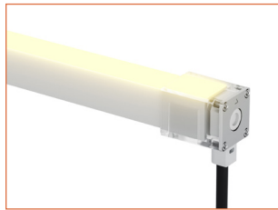
NF1617S-MEC-RB-2P Mechanical end cap with screws, right bottom entry, 11.8lin. (300mm) cable, 2 pin, IP67
