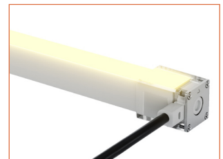
NF1617T-MEC-RS-2P Mechanical end cap with screws, right side entry, 11.81in. (300mm) cable, 2 pin, IP67
