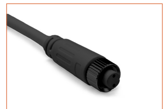
FCB-2P-67 Female connector, 11.8in. (300mm) black cable, 2 pin, IP67, Wet, 18 AWG
