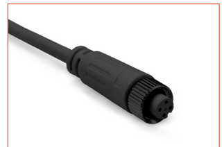
FCB-4P-67 Female connector, 11.8lin. (300mm) black cable, 4 pin, IP67, Wet, 18 AWG
