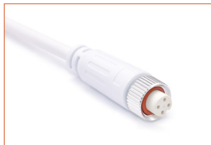
FCW-4P-67 Female connector, 11.8lin. (300mm) white cable, 4 pin, IP67, Wet, 18 AWG
