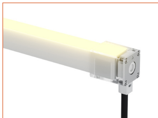
NF1617T-MEC-RB-4P Mechanical end cap with screws, right bottom entry, 11.81in. (300mm) cable, 4 pin, IP67
