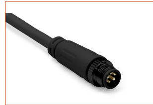
MCB-5P-67 Male connector, 0.98ft (30cm) black cable, 5 pin, IP67, Wet, 22 AWG
