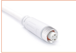
FCW-5P-67 Female connector, 11.8in. (300mm) white cable, 5 pin, IP67, Wet, 22 AWG
