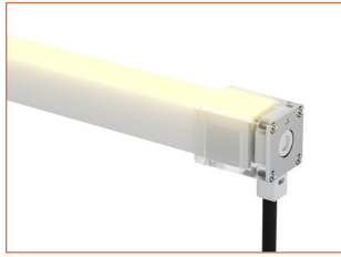
NF1617S-MEC-RB-5P Mechanical end cap with screws, right bottom entry, 11.8lin. (300mm) cable, 5 pin, IP67
