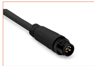
MCB-5P-67 Male connector, 11.81in. (300mm) black cable, 5 pin, IP67, Wet, 20 AWG
