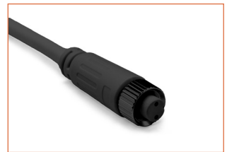
FCB-2P-67 Female connector, 11.81in. (300mm) black cable, 2 pin, IP67, Wet, 20 AWG
