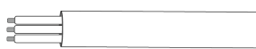
OW: Open wire, Dry only Standard 11.8in. (300mm), 18 AWG, wire length customizable
