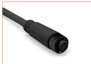
FCB-5P-67 Female connector, 11.8in. (300mm) black cable, 5 pin, IP67, Wet, 20 AWG
