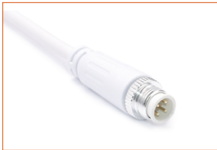
MCW-4P-67 Male connector, 11.8lin. (300mm) white cable, 4 pin, IP67, Wet, 20 AWG
