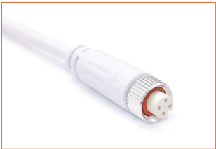
FCW-4P-67 Female connector, 11.8lin. (300mm) white cable, 4 pin, IP67, Wet, 20 AWG
