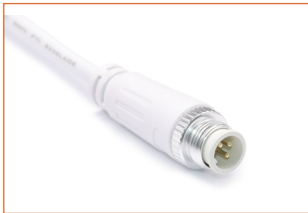
MCW-3P-67 Male connector, 11.8lin. (300mm) white cable, 3 pin, IP67, Wet, 20 AWG
