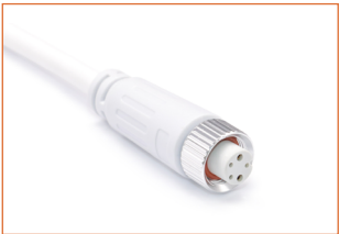
FCW-5P-67 Female connector, 11.8lin. (300mm) white cable, 5 pin, IP67, Wet, 20 AWG
