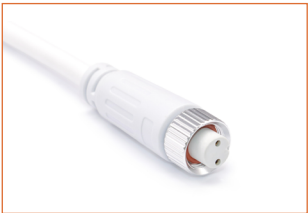
FCW-PU-2P-67 Female connector, 11.8lin. (300mm) white PU cable, 2 pin, IP67, Wet, 20 AWG
