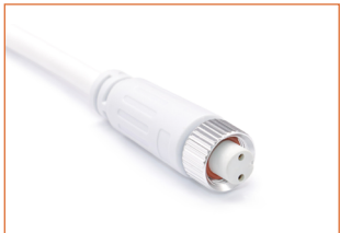
FCW-2P-67 Female connector, 11.8lin. (300mm) white cable, 2 pin, IP67, Wet, 20 AWG
