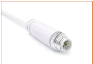
MCW-2P-67 Male connector, 11.8lin. (300mm) white cable, 2 pin, IP67, Wet, 20 AWG
