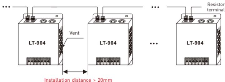
RJ45 connected in parallel
