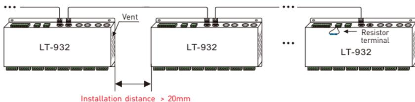
RJ45 connected in parallel
