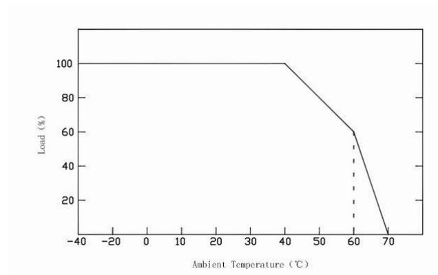
\*To ensure the driver's long life, please refer to the Derating Curve and derate according to the ambient temperature.
