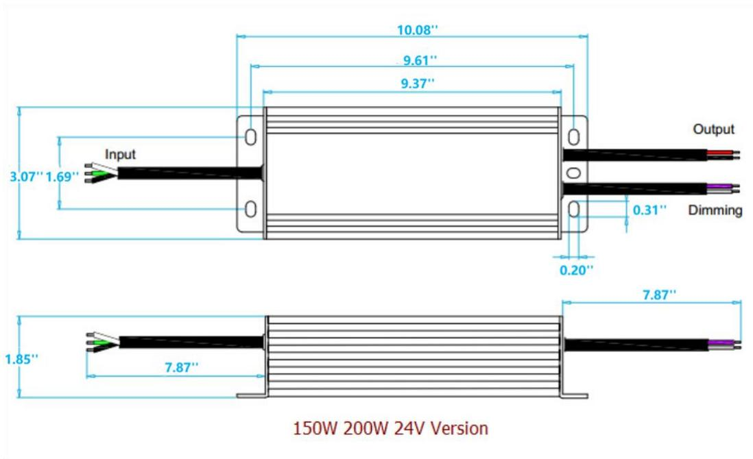
1. The input terminal has a 3-pin wire, of which the green wire is to be connected to the ground, black and white connected to AC L and N.
