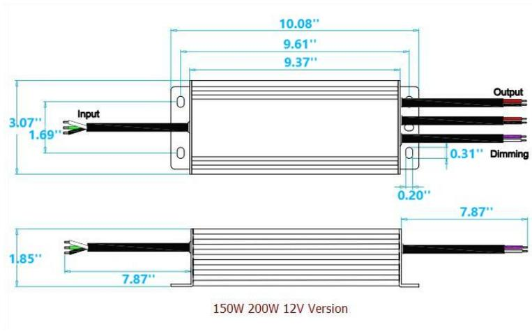
1. The input terminal has a 3-pin wire, of which the green wire is to be connected to the ground, black and white connected to AC L and N.
