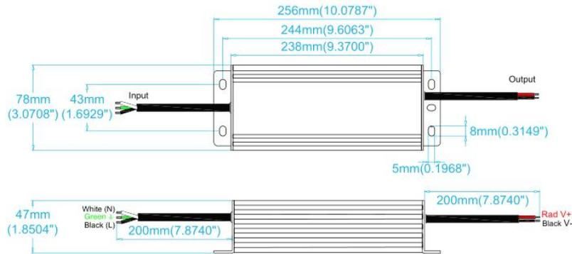
1. The input terminal has a 3-pin wire, of which the green wire is to be connected to the ground, black and white connected to AC L and N.
