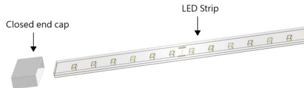
**Step 1** Peel off a small section of 3M tape on the back of the tape to install closed end cap.
