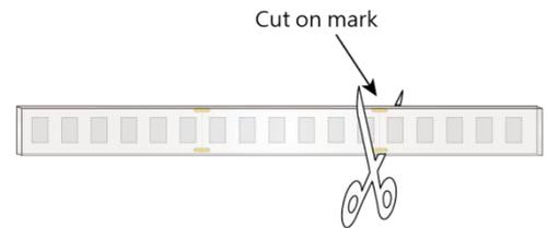
**Step 2** Use factory-recommended cutter, gently cut straight down through the body of the product directly on the cutting increment mark. DO NOT cut diagonally or horizontally as this may damage the product.
