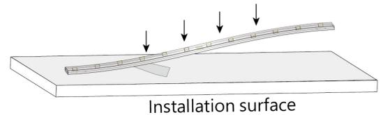
**Step 3** Gently press the tape back and forth to make sure that it's flat and firm without any air pockets.
