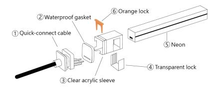
*Step 1* Push the clear acrylic sleeve to wrap around the neon.
