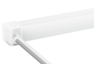
LN0606-SEC-S-2P Silicone end cap side entry with 0.98' (30cm) cable, 2 pin
