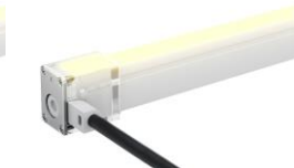
LIN1220-MEC1-LS-3P Mechanical end cap with screws, left side entry with 0.98' (30cm) cable, 3 pin
