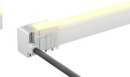
LIN1220-MEC3-LS-3P Mechanical end cap without screws, left side entry with 0.98' (30cm) cable, 3 pin
