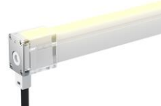
LIN1220-MEC1-B-3P Mechanical end cap with screws, bottom entry with 0.98' (30cm) cable, 3 pin
