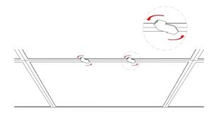
Step 4 Align the LED strip with attached connectors to the magnetic bases on your installation surface. Gently push upward until the magnets connect. The magnetic design allows for easy installation and removal for maintenance.
