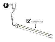
Step 2 Determine the desired location and lengths of neon to be installed. Leave enough distance for power cable to reach the power supplies.
