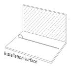
**Step 3** Install the adjustable clips into position with screws. It is recommended to use ONE mounting clip for 1 ft of the neon.
