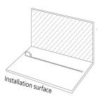
Step 3 Determine the locations and quantity of the mounting clips based on the information from Step 1. It is recommended to use ONE mounting clip for 1 ft of the neon.
