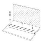
Step 4 Gently push the neon into the channel at the beginning of the run with palm instead of fingers and moving down the line towards the end.
