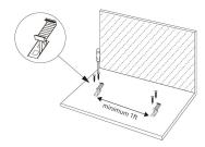
**Step 4** Install the adjustable clips with mounting channel by pushing them into the groove of the adjustable clips.
