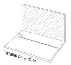
Step 3 Install the channel into position with screws. Make sure the screw head is flush or lower the base of the channels. DO NOT screw at an angle.
