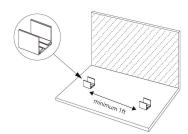
Step 4 Install the mounting clips into position with screws. Make sure the head is flush or lower the base of the channels. DO NOT screw at an angle.
