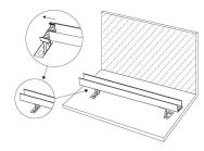
Step 5 Gently push the neon into the mounting channel from one direction with palm instead of finger.
